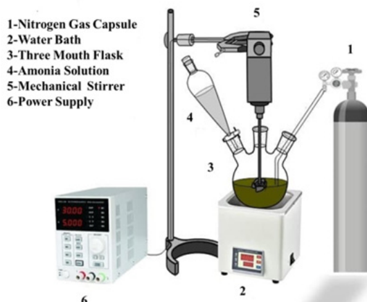
Figure 1. Schematic of the synthesis system of magnetic iron oxide ( \text{Fe}_3\text{O}_4 ) by co-precipitation method
